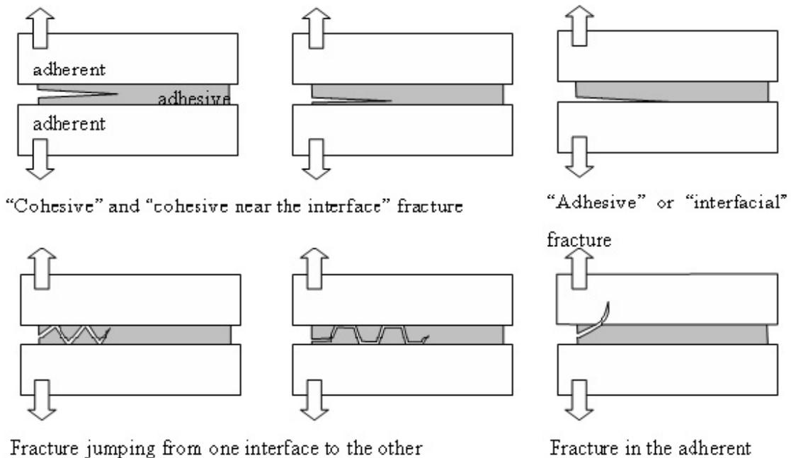
Figure 4.1 – Adhesive Failure Modes (from <http://wikipedia.org>)
