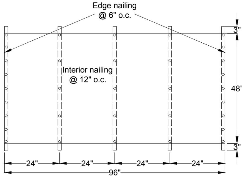
Figure 3.1 – Test Specimen Layout and Fastening Schedule
