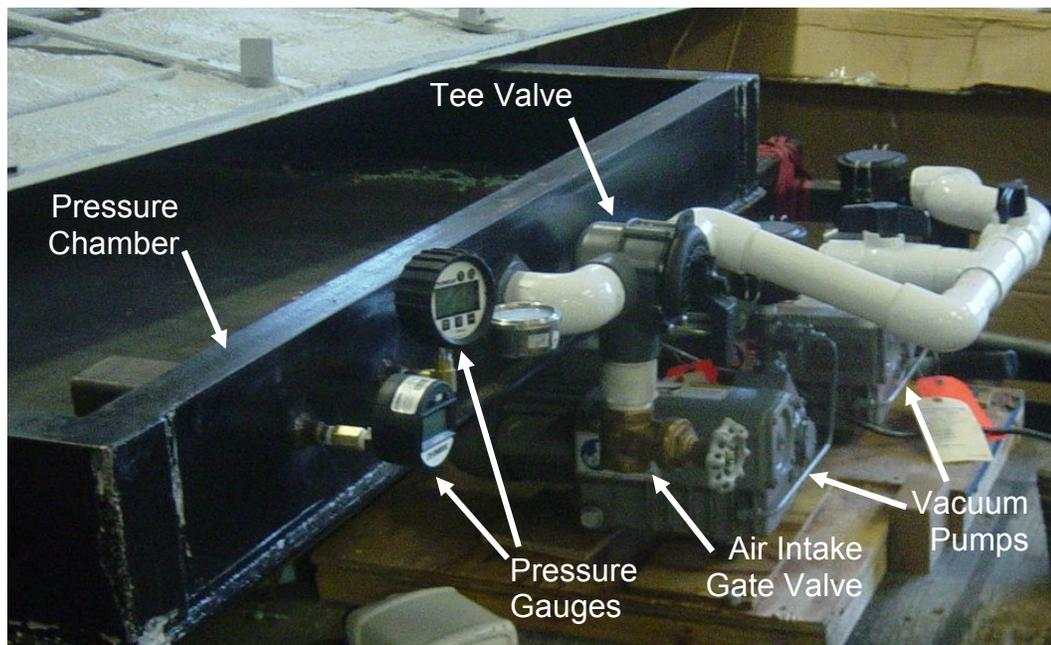
Figure 3.2 – Pressure Chamber, Vacuum Pumps and Controls
