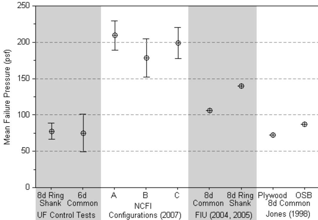
Figure 6.1 – Mean Uplift Capacities of Roof Panel Specimens from NCFI Tests Compared with Previous Results (Horizontal ticks indicate the 95% confidence interval of mean failure load)
