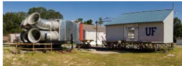
Figure 12: Hurricane Simulator at University of Florida
