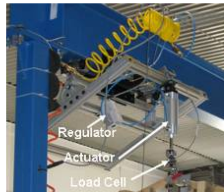
Figure 8: Load actuator setup
