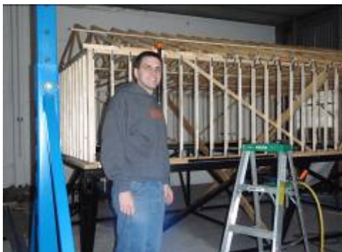
Figure 5: 1/3-scale house framing
