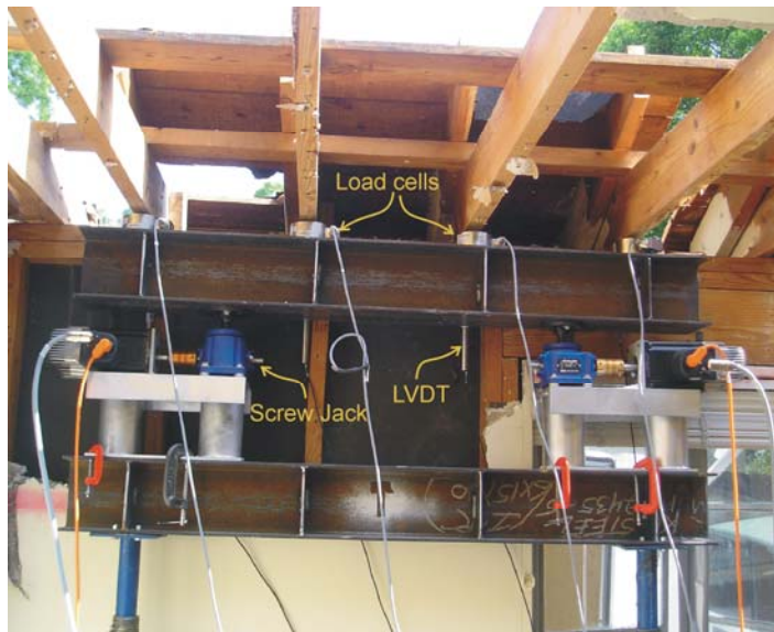
FIGURE 4 EXPERIMENTAL SET UP FOR UPLIFT TESTS
