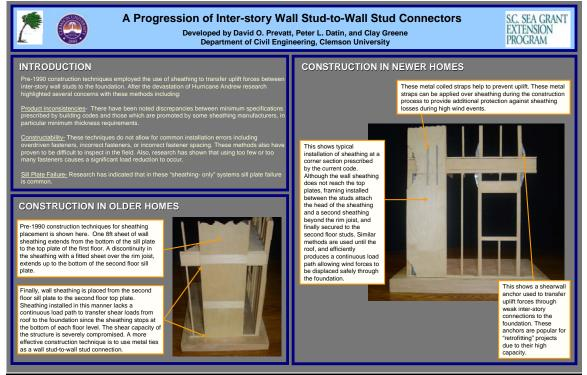
Figure 2: Development of Inter-story Ties in Wood Construction
