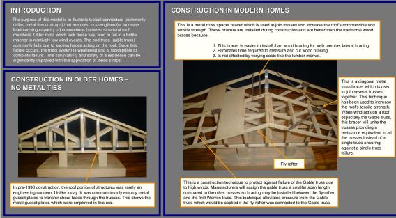
Figure 4: Hurricane Resistant Roof Construction Techniques
