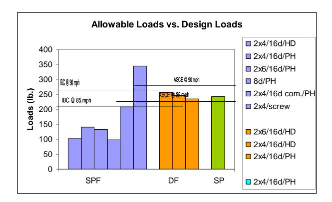
Figure 1: Tested allowable loads versus Allowable design loads
