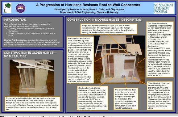
Figure 1: Hurricane Resistant Roof to Wall Connections
