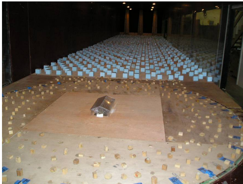
Figure 2.2 – Wind tunnel arrangement for 1:50 suburban terrain
