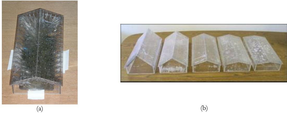
Figure 2.4 – (a) 4 in 12 sloped gable roof model used for this study and (b) The entire Clemson Standard Model (CSM) set
